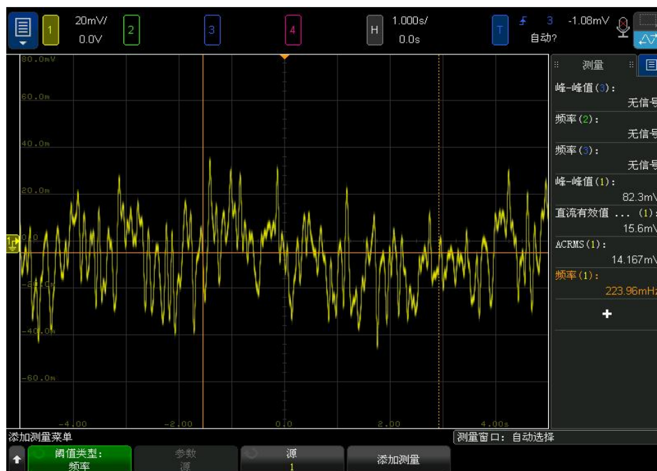
Figure 3 Voltage noise image (100,000x magnification)
